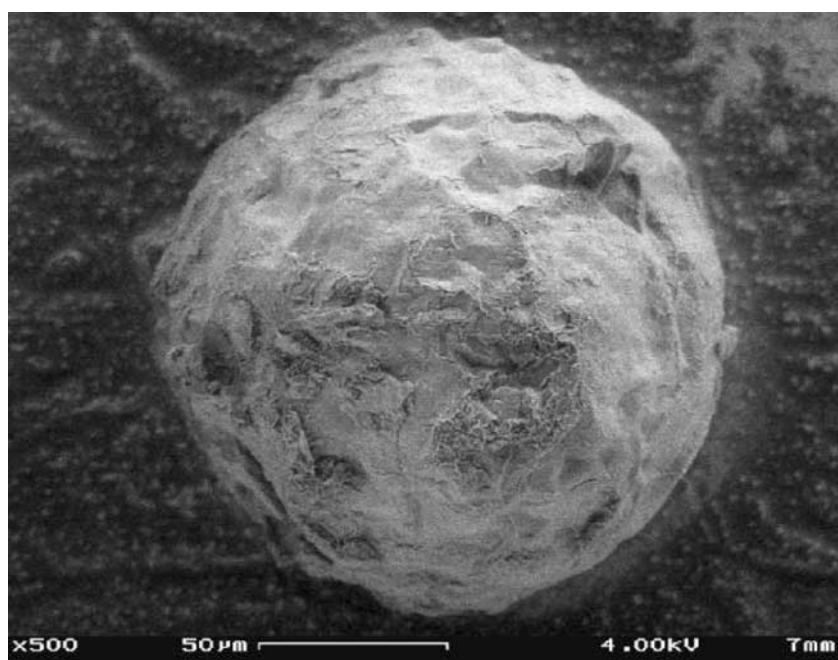
Figure 3. Scanning electron micrograph of microspheres with colloidal silica.
